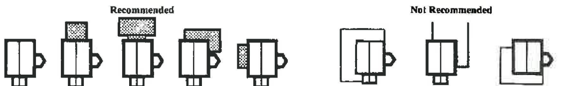
Compatible locations for additions. Setback from the original house so less visible and smaller in scale
