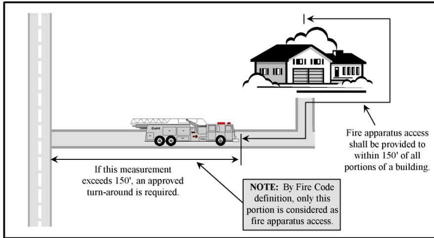
**DEAD END ROADS:** Dead end fire apparatus access roads in excess of 150 feet in length shall be provided with an approved turnaround. Diagrams of approved turnarounds are shown below: (OFC 503.2.5)
