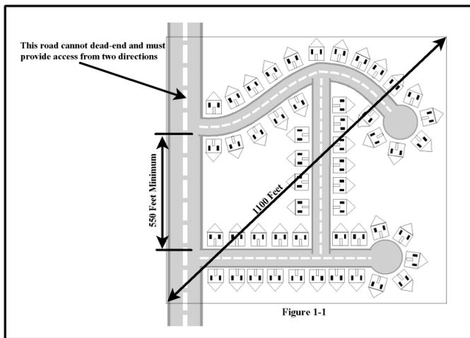
**FIRE APPARATUS ACCESS ROAD WIDTH AND VERTICAL CLEARANCE:** Fire apparatus access roads shall have an unobstructed driving surface width of not less than 20 feet (26 feet adjacent to fire hydrants (OFC D103.1)) and an unobstructed vertical clearance of not less than 13 feet 6 inches. (OFC 503.2.1 & D103.1)
