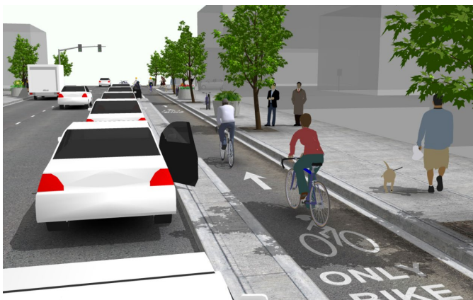
Figure 4. One-Way Separated Bike Lanes: Protected Bike Lane (left) - NACTO Urban Bikeway Design Guide Buffered Bike Lane (right) – City of Corvallis, Oregon
