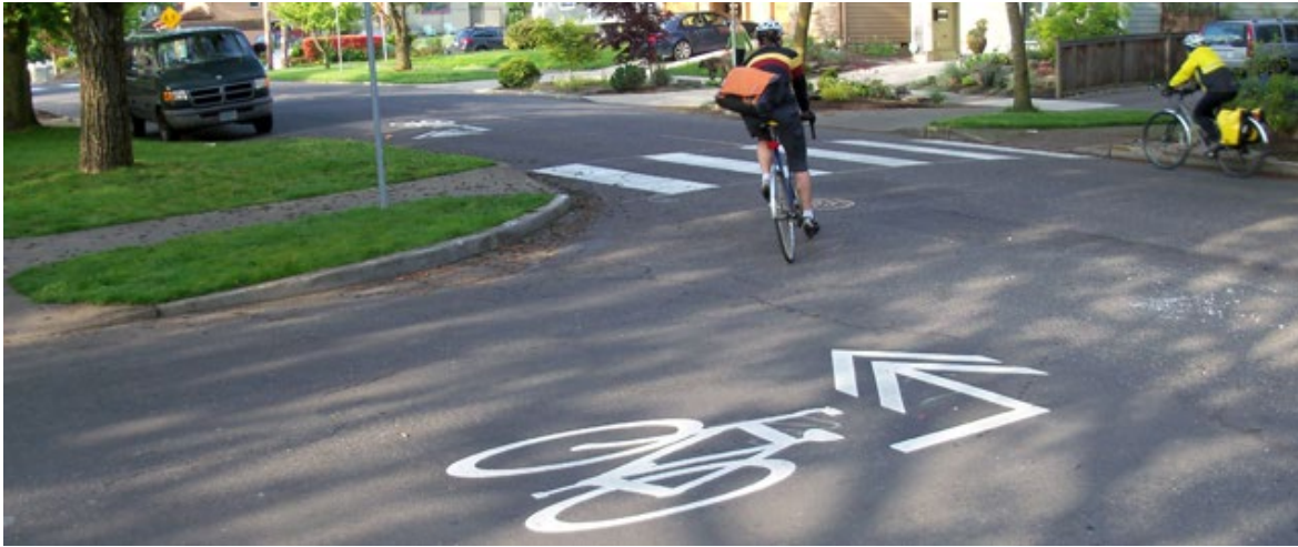
Figure 13. Wayfinding Using Sharrows - NACTO Urban Bikeway Design Guide
