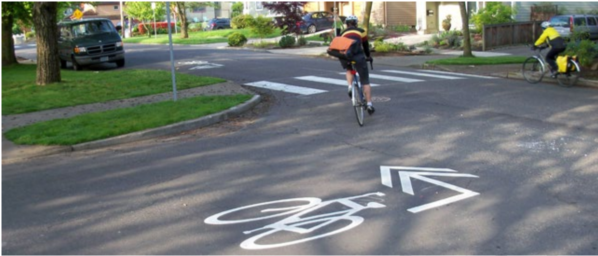
Figure 12. Wayfinding Using Sharrows - NACTO Urban Bikeway Design Guide
