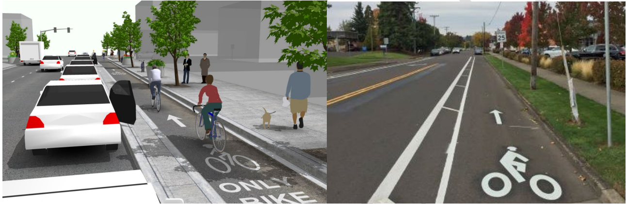
Figure 4. Class 2 Bikeways: Protected Bike Lane (left) - NACTO Urban Bikeway Design Guide Buffered Bike Lane (right) – City of Corvallis, Oregon
