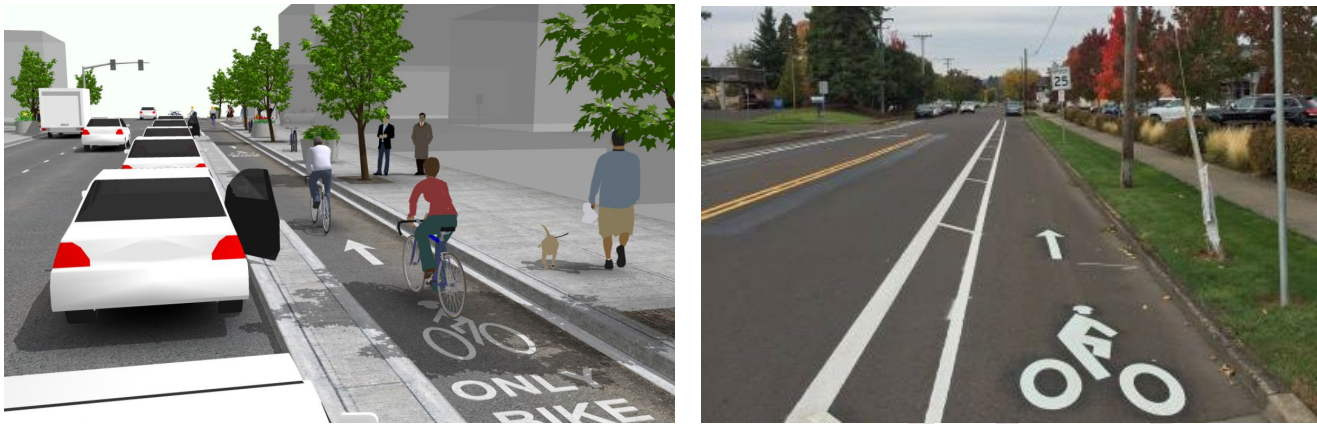
Figure 3. One-Way Separated Bike Lanes: Protected Bike Lane (left) - NACTO Urban Bikeway Design Guide Buffered Bike Lane (right) – City of Corvallis, Oregon
