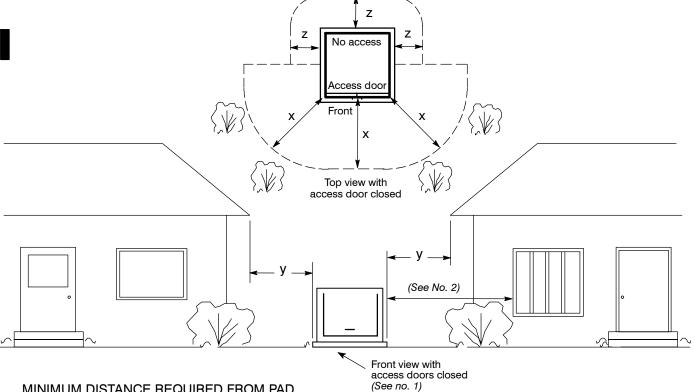
Figure 5.5 - Padmounted Equipment Clearances
