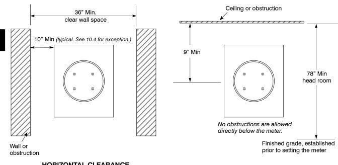
Figure 5.1.1 - Meter Socket Clearance Requirements
