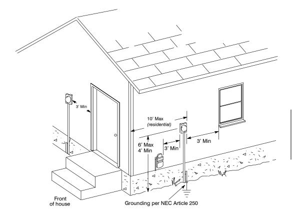
Figure 5.2.2 - Clearances for Underground Service
