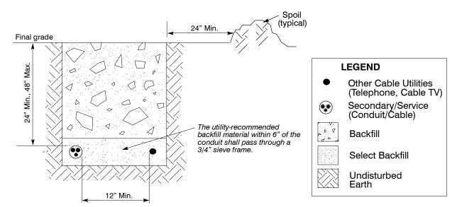
Figure 6.3.4 - Joint Use Service Trench
