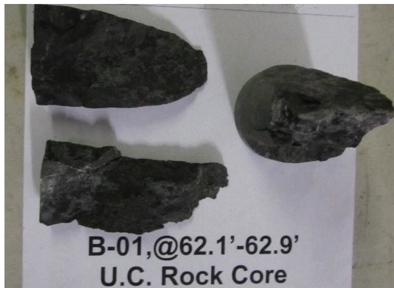
Figure 8. B-1 @ 62.1 – 62.9 Ft. core after unconfined strength testing.
