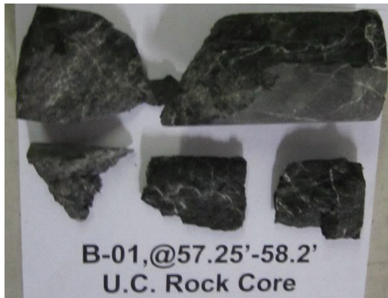
Figure 6. B-1 @ 57.3 – 58.2 Ft. core after unconfined strength testing.
