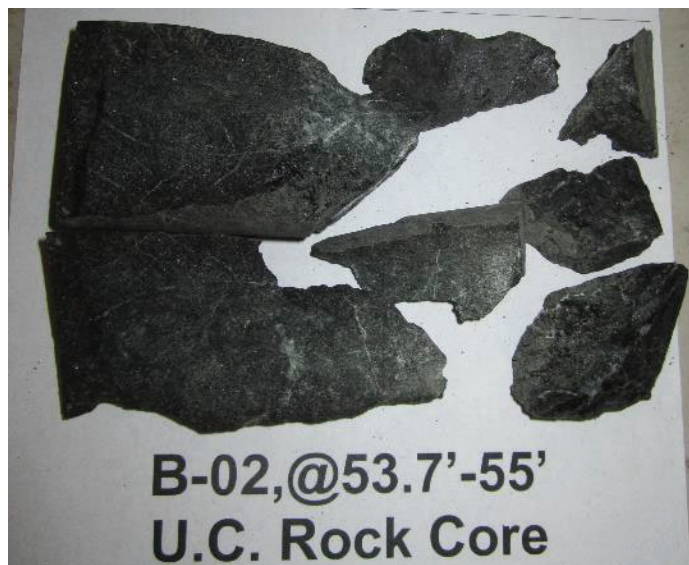
Figure 16. B-2 @ 53.7 – 55.0 Ft. core after unconfined strength testing.
