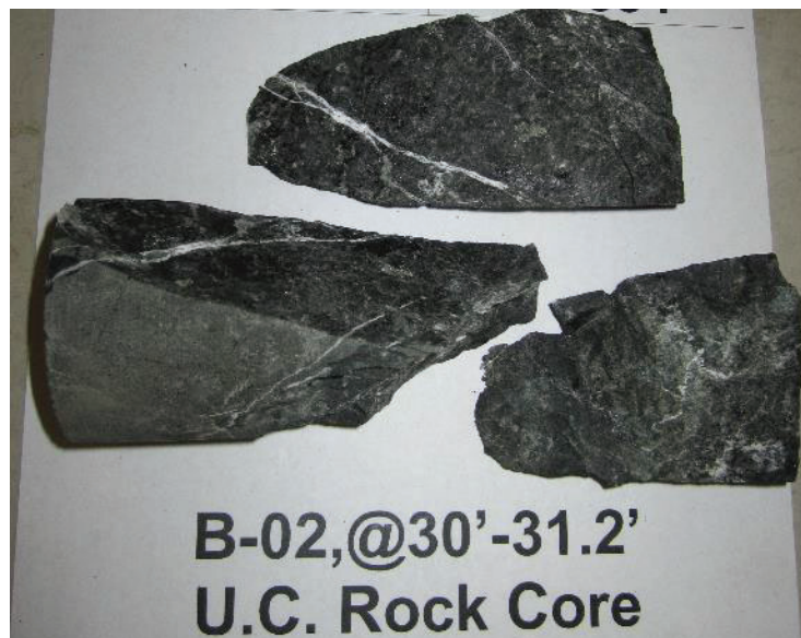
Figure 12. B-2 @ 30.0 – 31.2 Ft. core after unconfined strength testing.
