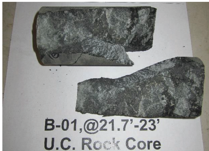
Figure 2. B-1 @ 21.7 – 23.0 Ft. core after unconfined strength testing.
