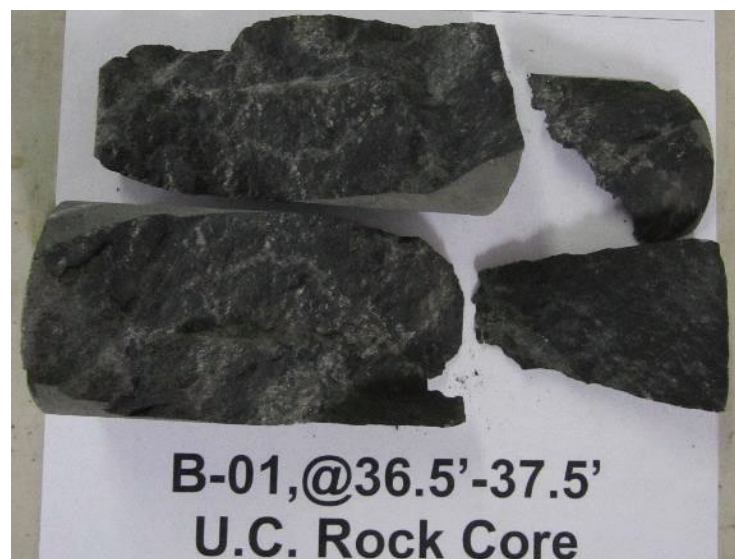
Figure 4. B-1 @ 36.5 – 37.5 Ft. core after unconfined strength testing.
