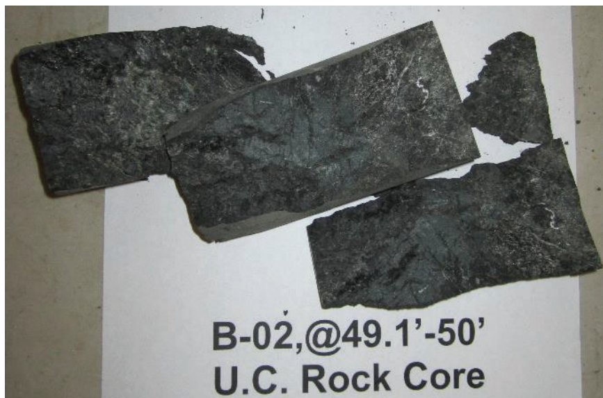
Figure 14. B-2 @ 49.1 – 50.0 Ft. core after unconfined strength testing.
