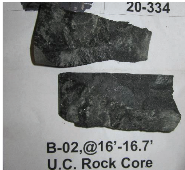
Figure 10. B-2 @ 16.0 – 16.7 Ft. core after unconfined strength testing.
